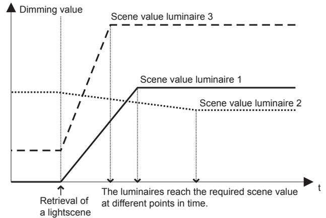
The "Same dimming time" function can be used to synchronise the different dimming times of the channels in such a way that all channels reach their set value at the same time. Using the "Time factor modifiable via the bus" parameter (via the communication object "Factor same dimming time"), the dimming times can also be synchronised for several dimming actuators.
