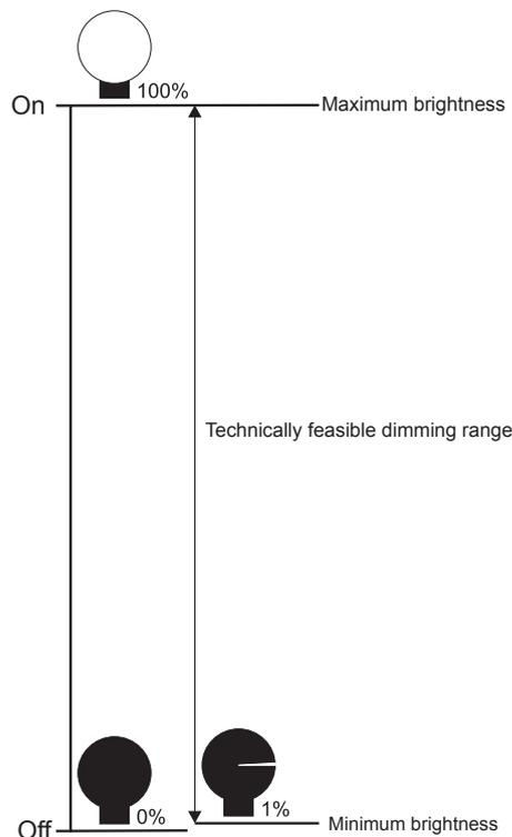
The dimming range which is technically possible can be limited using the software application to a minimum and a maximum dimming value. This limitation can be set individually for each output channel.
