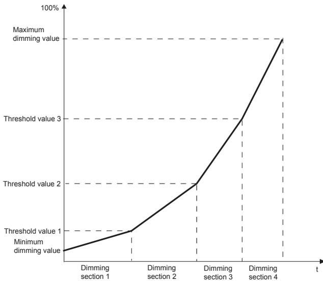
**i** The dimming hardware requires at least 500 ms to run through the entire dimming range from 0% to 100%. Please observe this limit value when setting the dimming times for the individual dimming sections. Overall dimming times which are shorter than 500 ms cannot be executed by the hardware.
