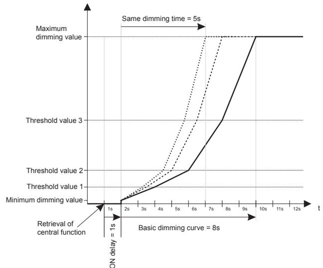
The ON delay is also retained with an identical dimming time. The dimming curve is compressed or extended in such a way that the dimming value is reached after the same dimming time. In other words, the calculation of the new dimming curve takes into account the pure dimming time (the same dimming time minus ON delay time).
