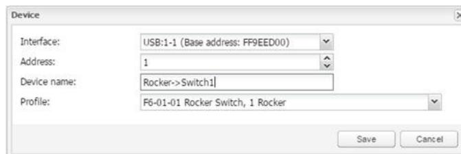
Once the device is added, pair it with specific device in EnOcean network. Set the EnOcean device in learning mode and then press Teach-in button in Wiser for KNX configuration.
