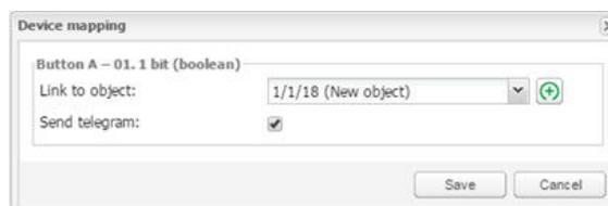
When KNX object value is changed (1/1/18 in the example above), telegram is sent to the device, which has been paired with Wiser for KNX virtual device (F6-01-01 in the example above).
