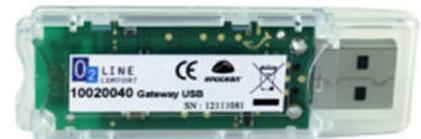
USB gateway is a small USB stick which connects PC's, consumer devices, DSL boxes and other USB master devices to EnOcean based radio products. It is equipped with a TCM 310 transceiver gateway module. It provides bidirectional EnOcean radio and bidirectional serial interface via USB. Radio messages are sent and received via an externally connected USB host.
